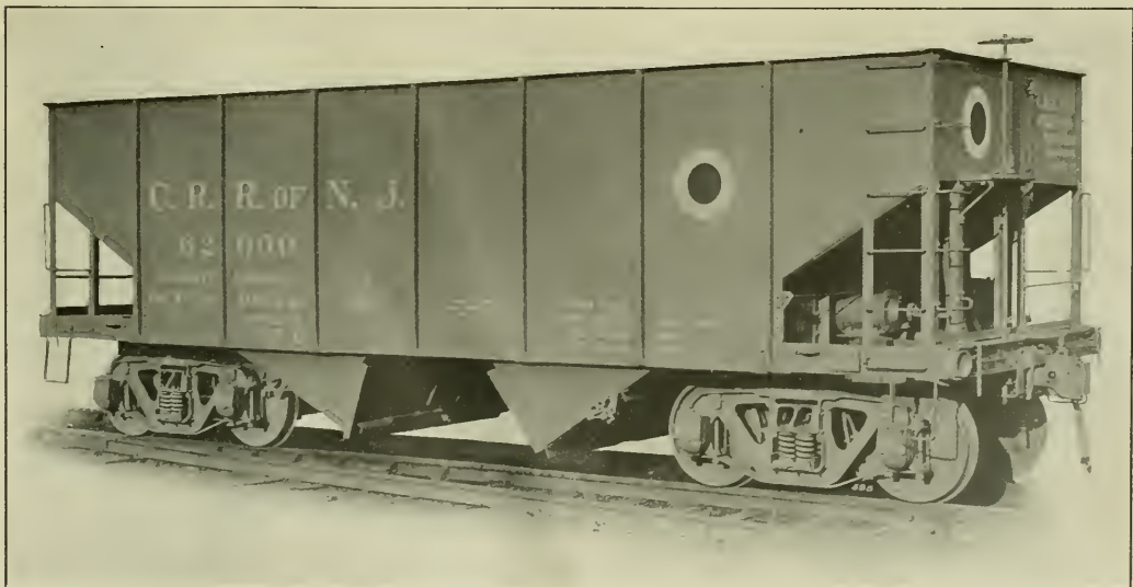
Latest Design of Steel Hopper Car on the Central Railroad of New Jersey.
